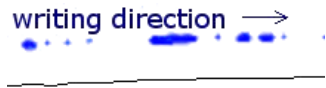
Figure 8: The direction of the closest stroke to the synchronization blob can be interpreted as the writing direction.
