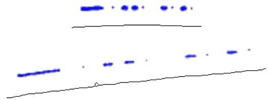
Figure 9: Different length of the n -pulse lines depending on the velocity. (top: slow velocity, bottom: faster velocity)
