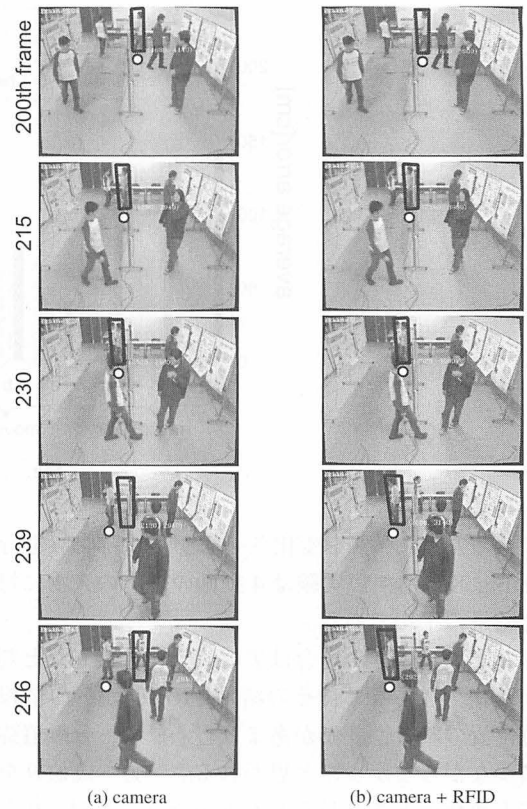
Fig. 6. Tracking result obtained when occlusion occurred. Rectangle: tracked position; circle: true position.
