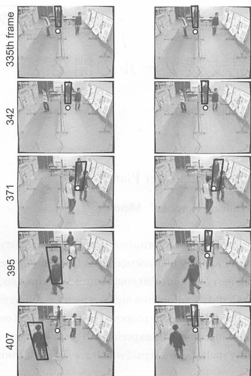
Fig. 9. Improvement by height information. Rectangle: tracking result. Circle: true position.
