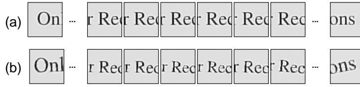
Fig. 2. Video frame sequence capturing a line of text. (a) Simple case. (b) General case.
