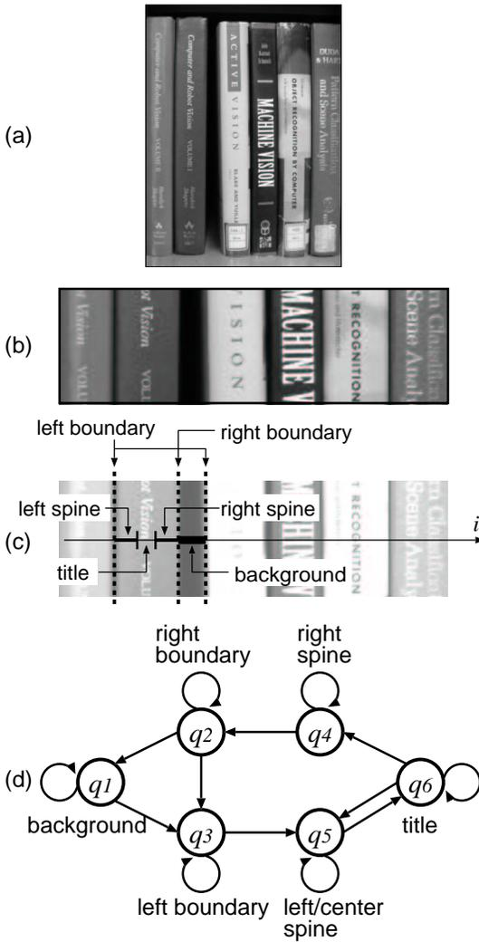
**Fig. 1.** (a) An original bookshelf image (HSI color image actually). (b) The middle part of (a). (c) The structural properties of (b). (d) An FSA representation of (c).
