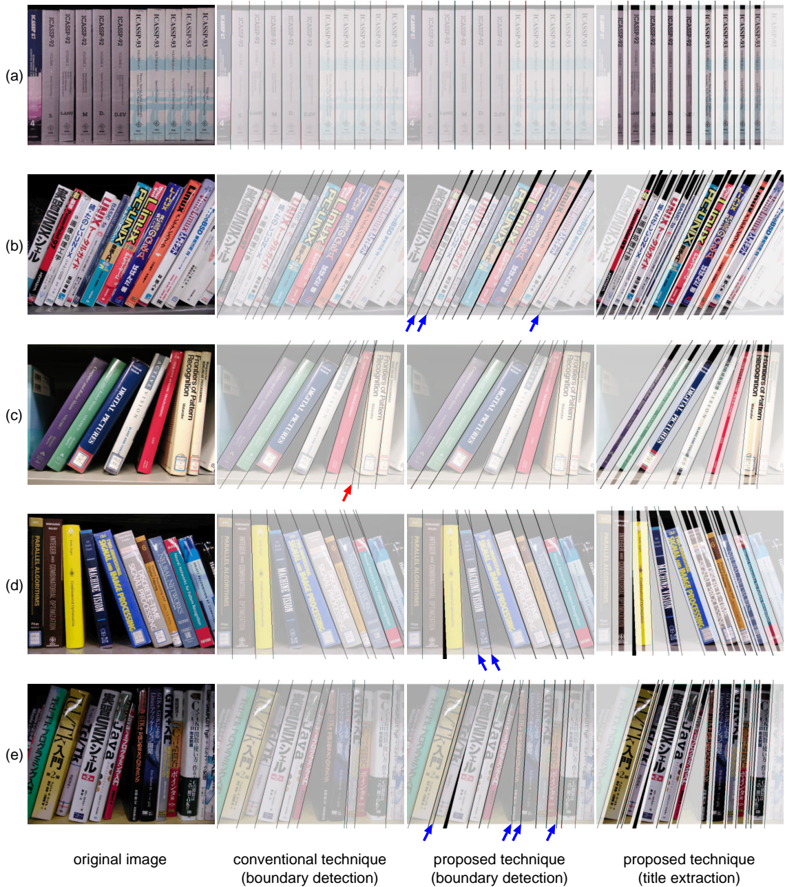
Fig. 6: Examples of book boundary detection and title extraction. From left to right: the original images, the results of the conventional boundary detection technique, the results of the first step of the proposed technique, and the results of the second step of the proposed technique. Book boundaries detected are shown as black lines. A spurious boundary is shown by a red arrow. Boundaries correctly detected only by the proposed technique are shown by blue arrows. In the results of the second step of the proposed technique, title parts extracted are non-shaded.
