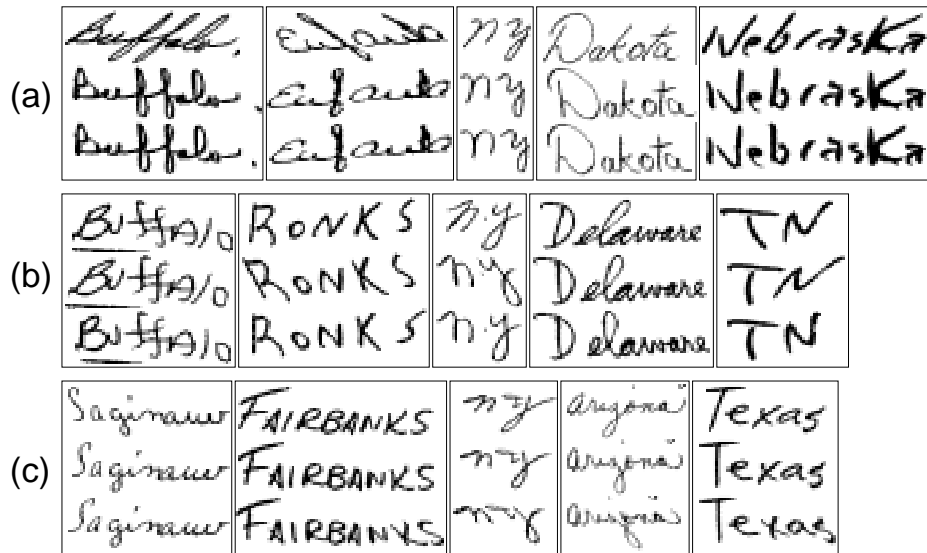
Figure 5. Examples of slant correction. For each word, the preprocessed image (top), the uniform slant correction result (middle), and the nonuniform slant correction result (bottom) are shown. The nonuniform slant correction results are similar (a), superior (b), and inferior (c), to the uniform slant correction results.
