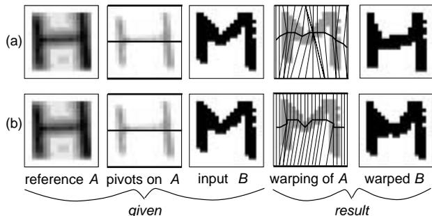
**Fig. 5. The effect of additional constraint: (a) excessive warping with conventional PL2DW, (b) suppression of excessive warping with the use of an additional local constraint.**
