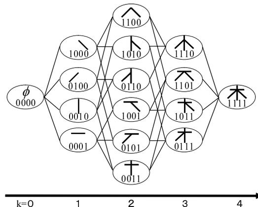
**Figure 4. Cube graph for optimal stroke correspondence to the reference pattern of four-stroke character “木” (“tree”). This cube graph also becomes a probabilistic one by embedding a stroke HMM and a probability  $p_{m,n}$  into each edge.**
