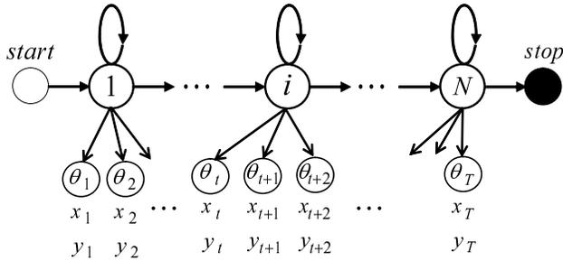
**Figure 1. A conventional HMM ( $\theta$ -HMM). At each state, a directional feature  $\theta_i$  is observed and a pen-coordinate feature  $xy_t = (x_t, y_t)$  is not.**
