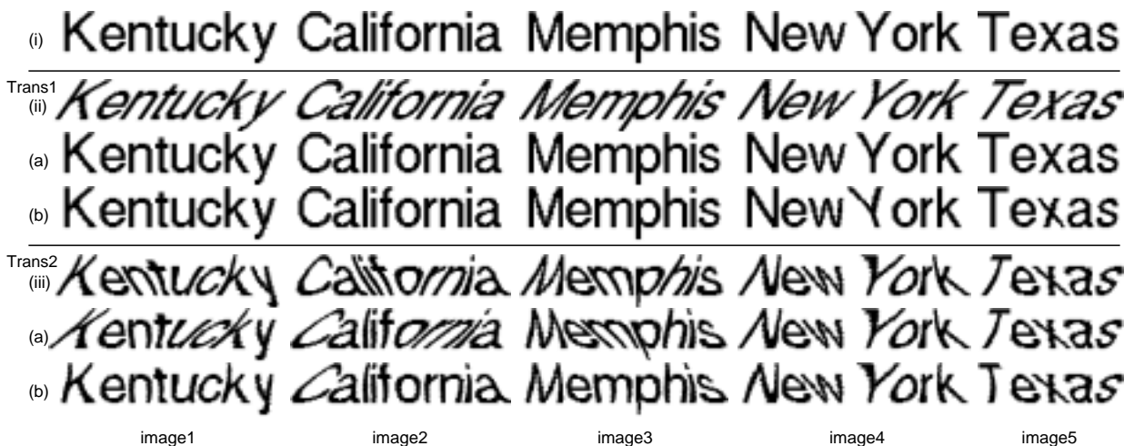
Fig.5 Slant correction for artificially slanted words by the conventional technique or the present technique.:(i)Original word images. (ii),(iii)Artificially slanted word images. (a)Slant corrected results of the conventional technique. (b)Slant corrected results of the present technique.
