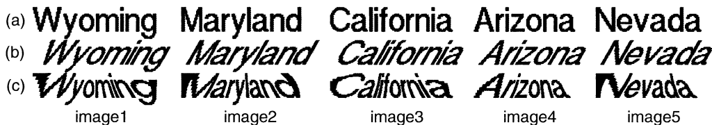
Fig. 7 Artificially slanted words. (a) Original image. (b) Slanted at the constant angle of 30°. (c) Nonuniformly slanted at angles sinusoidally changing in [-30°, 30°].
