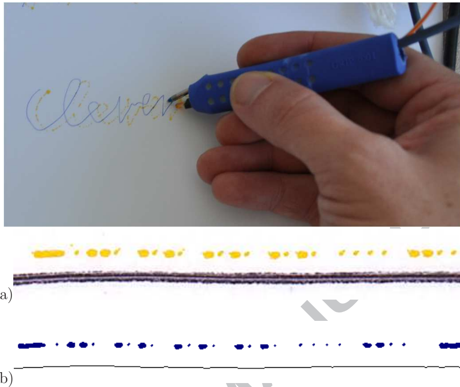
Figure 1: A prototype of the data-embedding pen (top). (a) Ink-dots (light) nearby a handwriting stroke (black). (b) After image processing.
