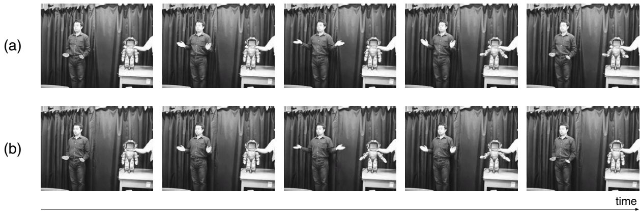
Figure 6. Result of delay compensation by the proposed prediction algorithm; the humanoid was driven by (a) delayed input posture and (b) the predicted posture.
